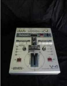
A photograph of the Edirol V-4 video mixer, a compact, light-colored device with various knobs, buttons, and a central fader. |
