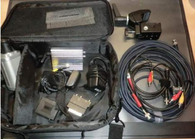
A photograph of the Sony surveillance camera kit, including the camera unit, a BNC cable, and other accessories in a carrying case.  |
